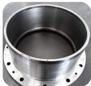
Stern Tube Bearing Sleeve Repair
