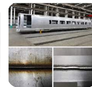
Laser Cleaning of Weld Oxides and Surface Contaminants
