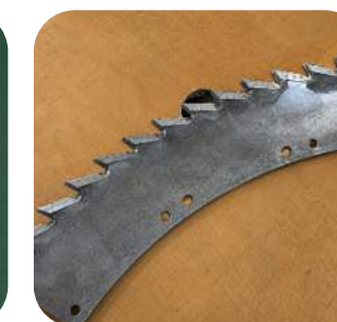
Pulverizer Blade Cladding
