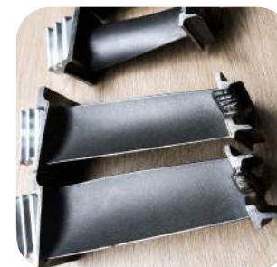
Low-Pressure Turbine Blade Repair
