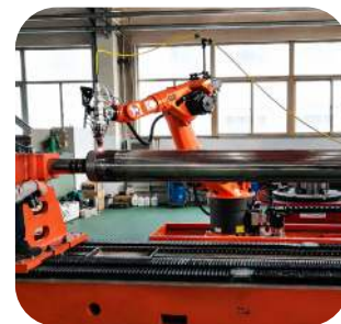
Piston Rod Repair
