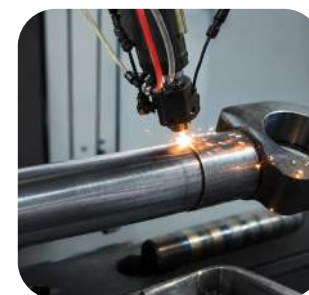
Piston Rod Repair
