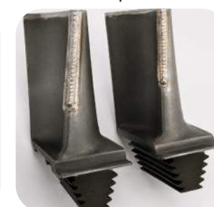
High-Pressure Turbine Blade Repair
