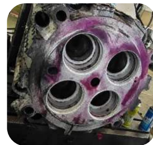
Diesel Engine Cylinder Head Repair
