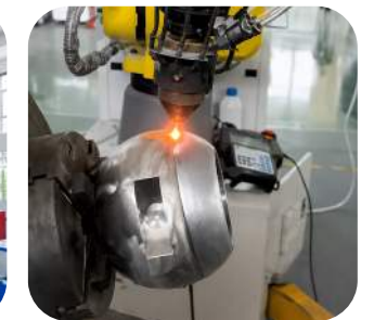
Ball Valve Laser Cladding
