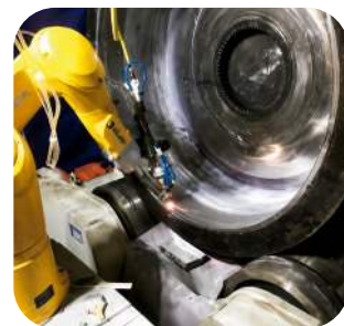
Overhead Crane Drum Inner Journal Repair
