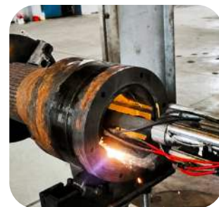
Fan Hub Sleeve Bore Repair
