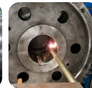
Gear Reducer Gear Repair
