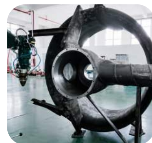
Stern Tube Repair
