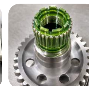
Spline Shaft Repair
