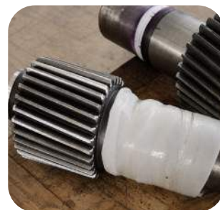
High-Speed Gear Laser Cladding Repair
