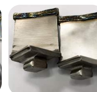
Compressor Blade Repair
