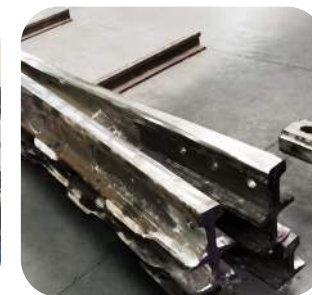
Railway Switch Frog Core Repair
