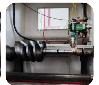
Compressor Screw Repair
