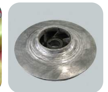
Hastelloy Impeller Repair
