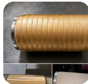
Babbitt Alloy Laser Cladding for Shaft Components
