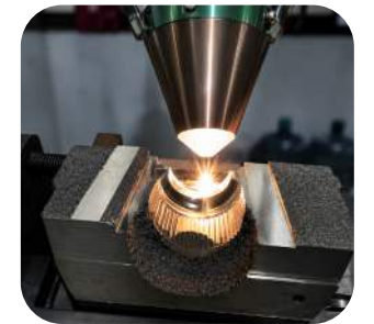
Glass Mold Repair
