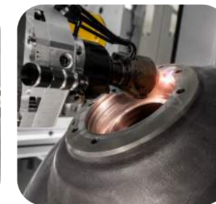
Traction Motor End Cover Repair
