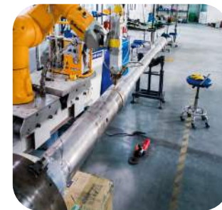
Long Shaft Wear Repair
