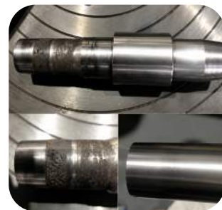
Pump Shaft Repair
