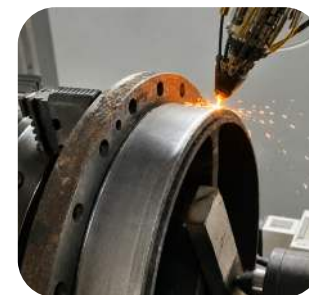
Shield Machine Bearing Sleeve Repair
