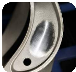
Gas Turbine Blade Build- Up
