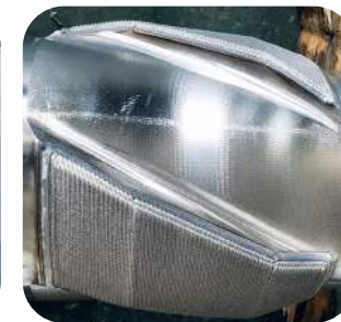
Centralizer Wear Repair
