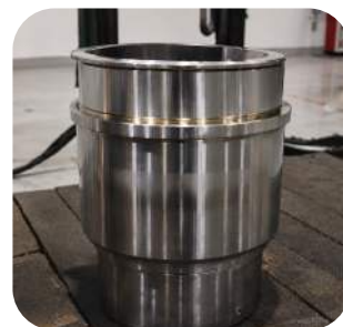
Intermediate Shaft Laser Cladding Repair
