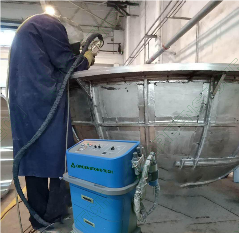
Cold Spray Repair of Aluminum Components
