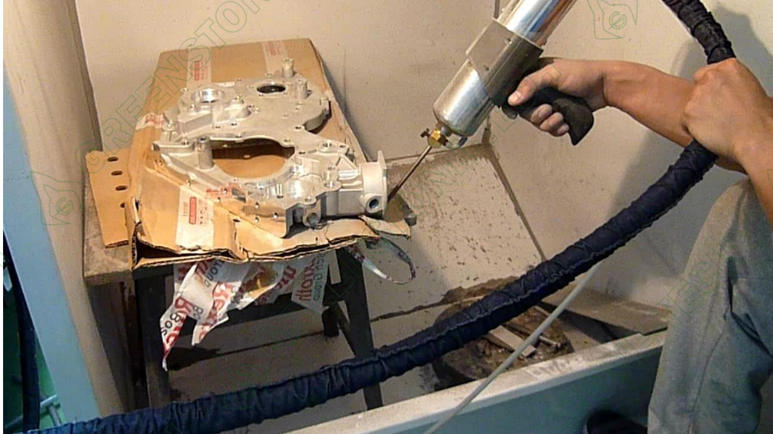
Cold Spray Repair of Aluminum Molds
