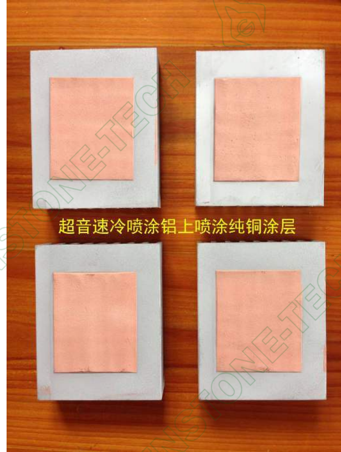
Supersonic Cold Spray - Pure Copper Coating on Aluminum
