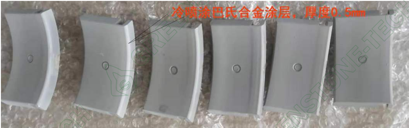
Deposition of Babbitt Alloy Coatings on Substrate Surfaces via Cold Spraying
